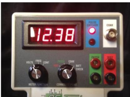
The top part of the tester is the test meter and is identical in both units. The lower part is specific to either valves or sensors. The testers have a super bright led display that is visible from 20 or more feet away from almost any angle. Meter functions are simple but fill the need. Measure 0 to 20 volts dc, frequency 0 to 1000hz, or resistance/continuity from 0 to 2000 ohms.
