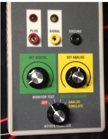
The HT101S is for digital and analog sensors. Digital sensors generate pulses at some frequency, Hz. They include flow meters, shaft speed sensors, and other movement sensors. Analog sensors include pressure and vacuum sensors, movement sensors, position sensors and so-on.
