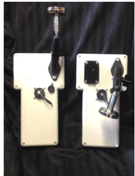
The testers then make those connected points available as “test jacks”. Ground and supply power is available along with the command wires for control valves or the signal line for sensors.
