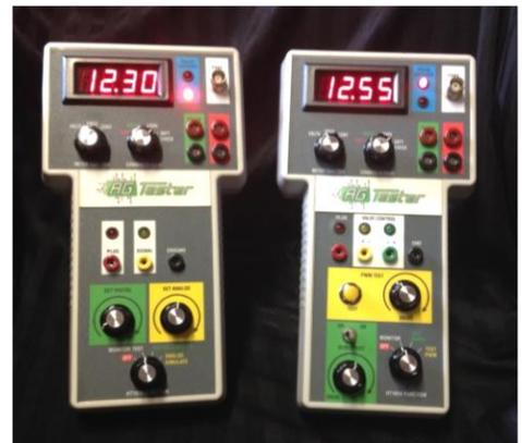
We have two hand-held testers that cover most any diagnostic need in the field. The HT101V will diagnose and fully test any valve on any machine. The HT101S will diagnose and fully test any sensor on any machine.
